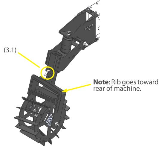
**3.1** - Pin new **Basket Insert (321592)** into **Basket Adapter (321590)** using **Pin (333099)** and securing with **Pin Clip (333021)**.
