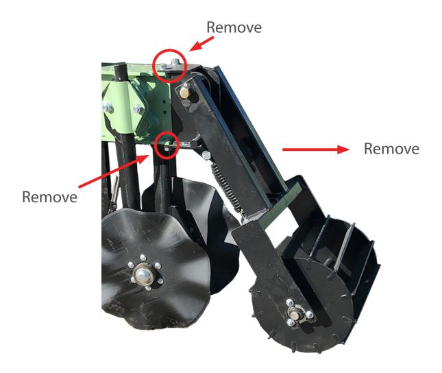
**1.1** - Using 3/4"Wrench and Rubber Mallet, carefully remove Orthman™ 1tRIPr™ Basket. All parts can be set aside and will NOT be reused.
