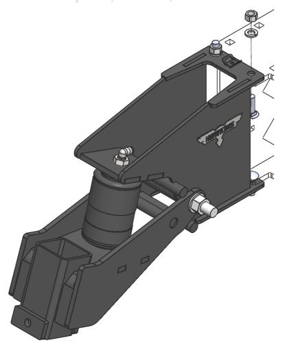
**2.1** - Using four (4) **Carriage Bolts (411785)**, four (4) **1/2" Lock Washers (413508)** and four (4) **1/2" Nuts (412058)**, attach the **Basket Adapter (321590)** to the 1tRIPr™ row unit.
