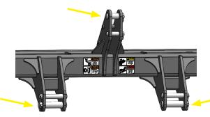
**2.** Once removed, the remaining pins are set to run the implement with a Category 3 hitch.
