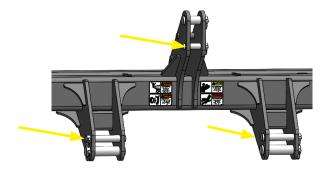
**2.** Once removed, the remaining pins are set to run the implement with a Category 4 hitch.
